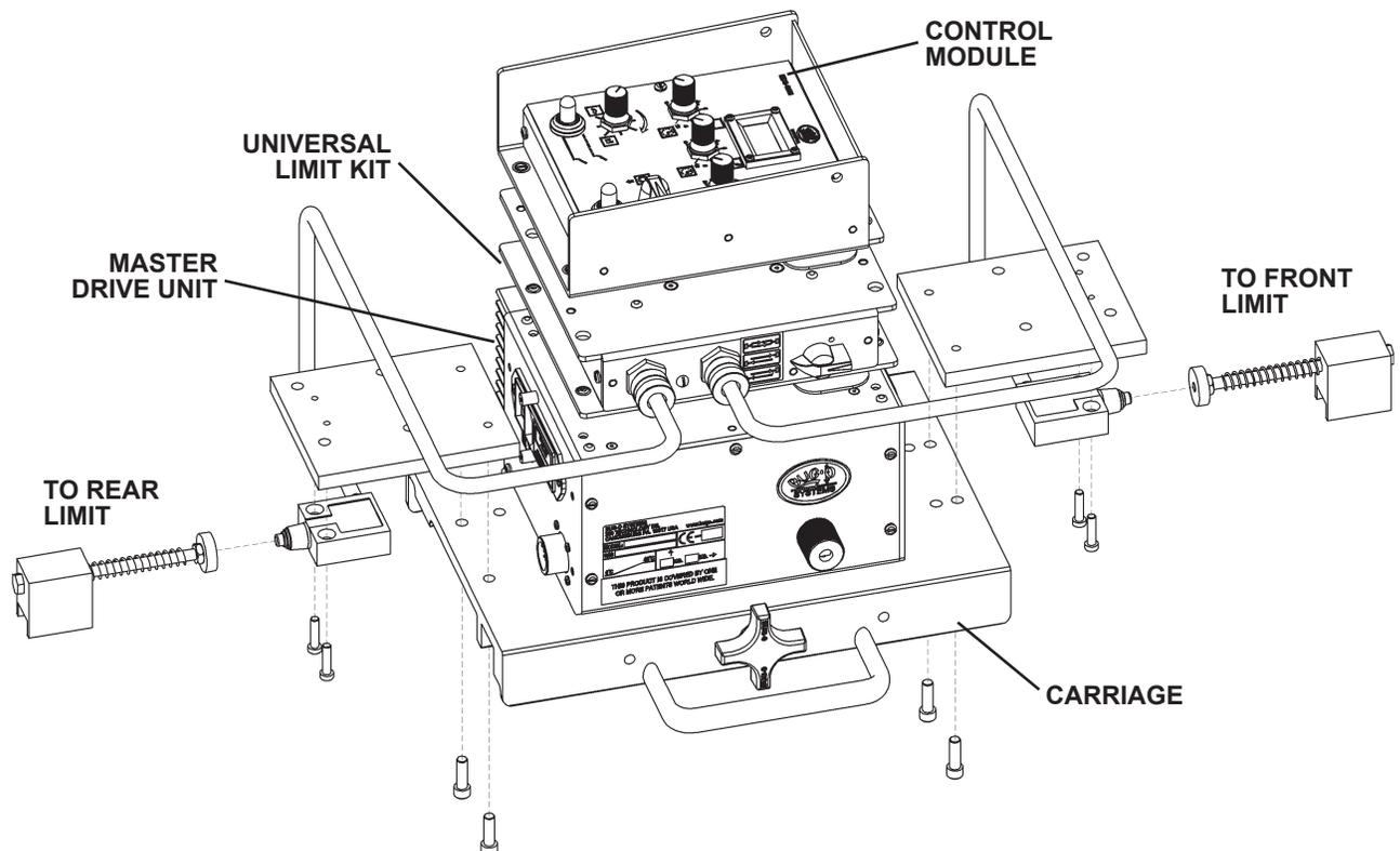
\* When using the MDS-1055 Universal Limit Kit with the MDS-1001 Straight Module, the Cycle Selector on the Straight Module must be set to **BASIC FORWARD/REVERSE** mode for the machine to operate. Use the mode selector on the MDS-1055 Universal Limit Kit to set the limit mode.
