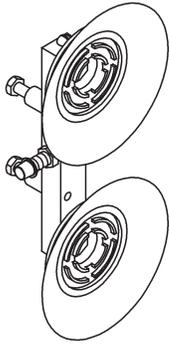
VACUUM CUPS are used for mounting the rail to the workpiece when magnet bars will not hold. EXAMPLE: Stainless steel or nonferrous surfaces. The surface must be smooth and nonporous.
