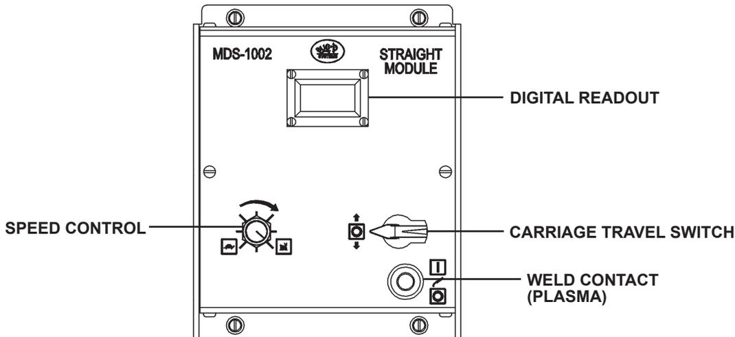
**SPEED CONTROL:** Sets the tractor speed from 2-120 in/min (5.1-304.8 cm/min).
