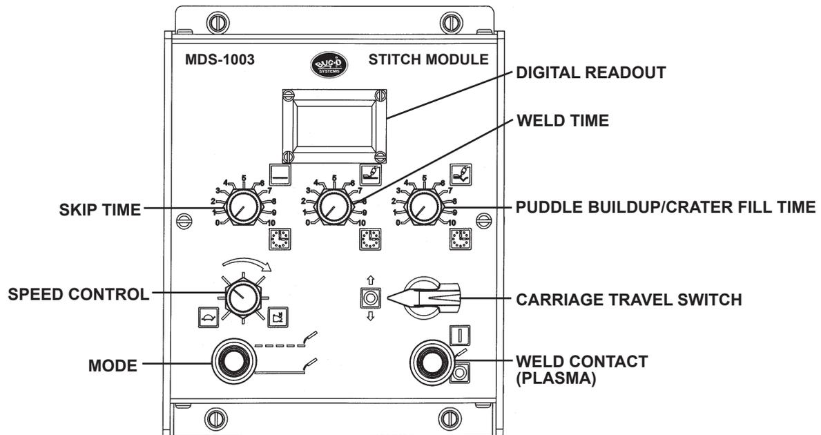
**SPEED CONTROL:** Sets the tractor weld speed from 2-120 in/min (5.1-304.8 cm/min).
