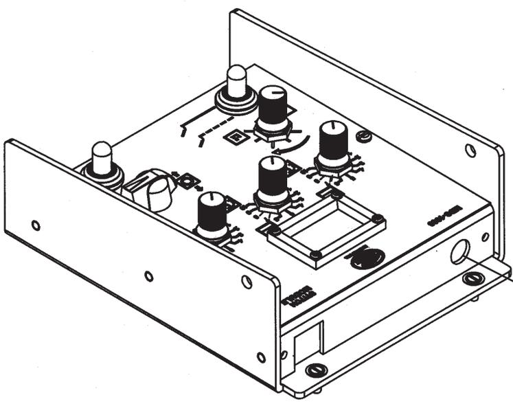
**STEP 4:** Set the speed display using a small slotted screwdriver.
