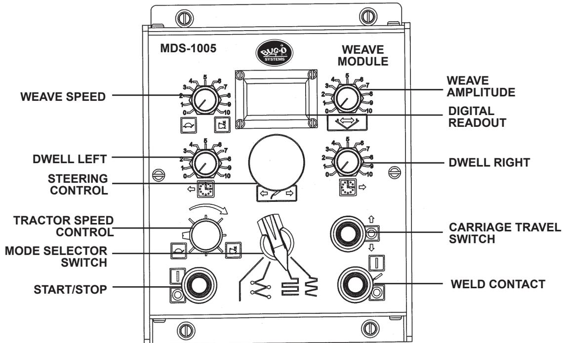
**AMPLITUDE (WEAVE):** Continuously adjustable up to a 2" (51 mm) maximum weaver stroke.
