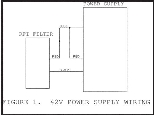
FIGURE 1. 42V POWER SUPPLY WIRING
