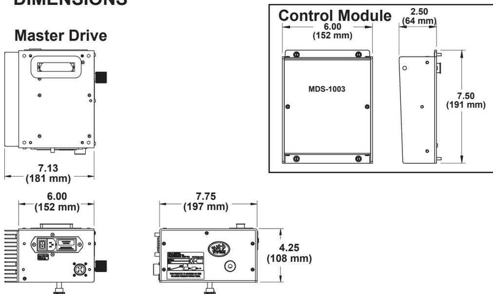
\*\* The Master Drive is rated at 60 lbs (27 kg) vertical load. The International Robotics Standards Rating requires a minimum of 2:1 continuous-duty safety margin on all power train and electronics components. The machine is equipped with overload protection.
