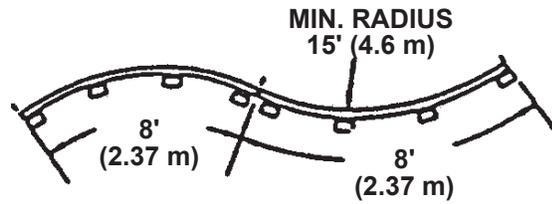
AFR-3000 FLEX RAIL replaces the old AFR-1000, 1010, 1020 and the later AFR-2000 rails. All the rack-mounting holes on the AFR-3000 Semi-Flex Rail are slotted so that the rack can slide along the rail. The length of the slots has been increased so that the rails can now be leapfrogged around a complete circle. The tension of the screws holding the rack on the rail is adjusted so that the rack can be moved along the rail with the AFR-2001 Rack-Adjusting Tool.
