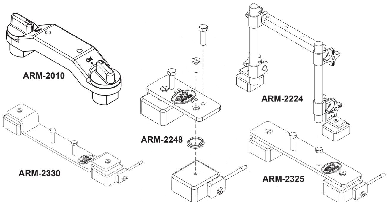
**NOTE:** Use four magnet assemblies per 8' (2.37 m) section and use two magnet assemblies per 4' (1.18 m) section.
