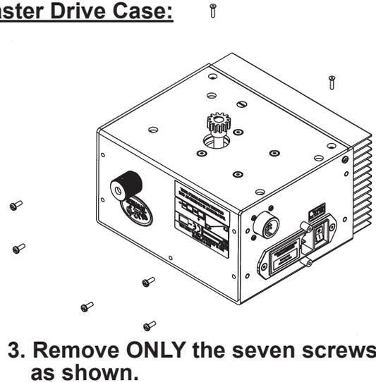
3. Remove ONLY the seven screws as shown.
