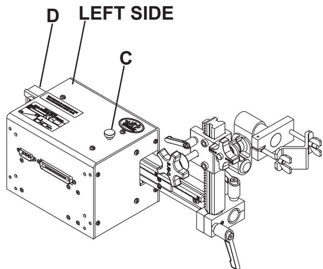
**CAUTION: IMPROPER GEAR MESH MAY CAUSE PINION, RACK, OR LINEAR WEAVER DAMAGE.**
