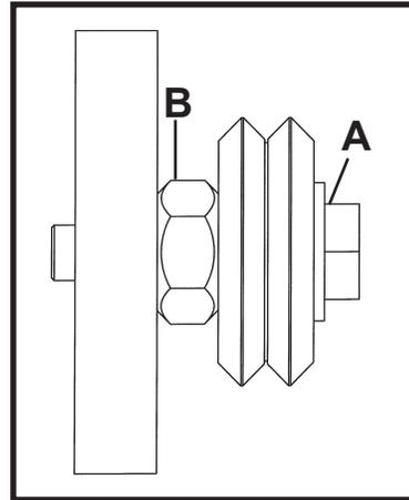
Check for proper alignment by using a finger to keep one of the wheels from rotating while manually moving the crossarm. The wheels are adjusted too tight if firm finger pressure is not enough to prevent wheel rotation. Once aligned, hold the adjustment bushing (B) still while tightening the hex bolt (A). Recheck alignment.
